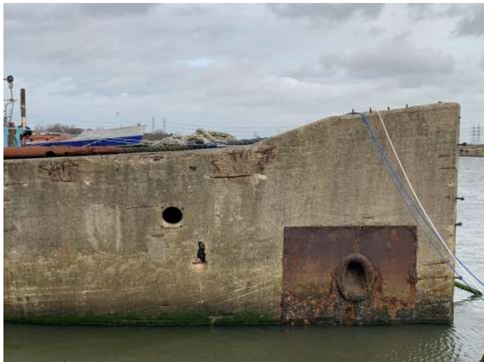
A fascinating close up of Violette showing its concrete structure taken more recently by Richard Lewis.
